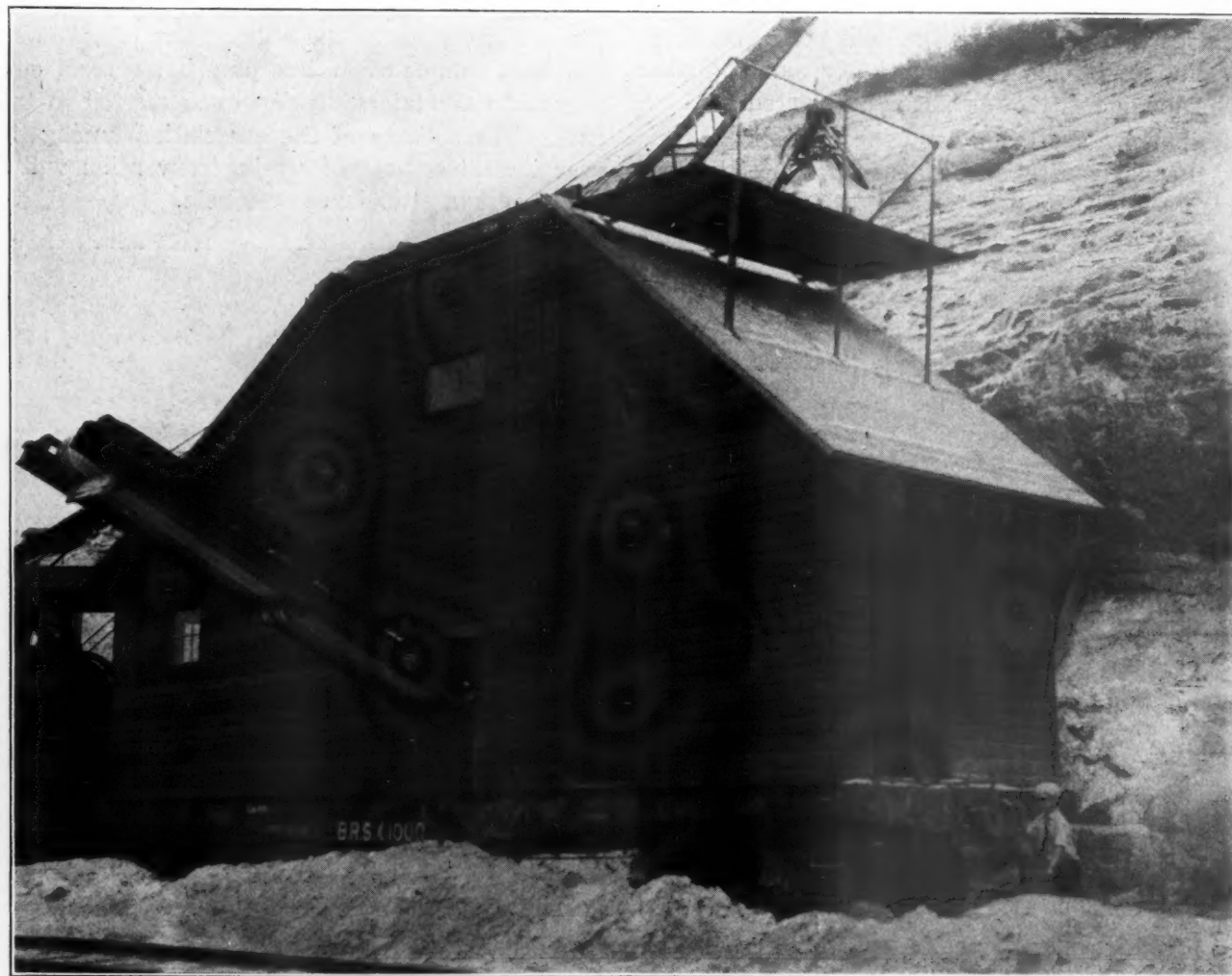
Close up of Portable Screening and Crushing Car
